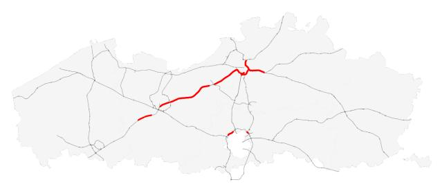
In the third stage of deployment, it seems rational for the ERS operator to extend the system to cover North-South axis on E17 on the route Antwerp-Lille, possibly starting from the border of Netherlands on E19 to Breda. Also, sections of E19 between Antwerp and Mechelen, the northern part of the Brussels ring road R0 and E40 could also be electrified.
