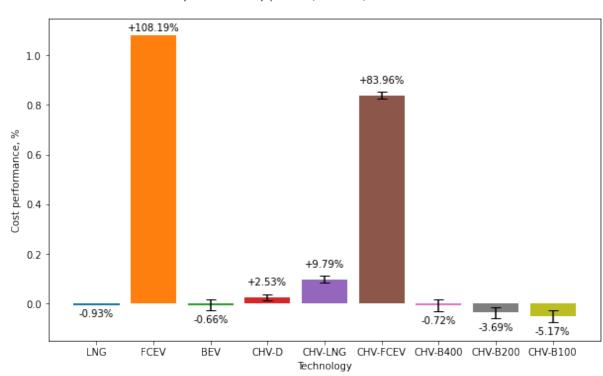
Figure 22 – Total technology vkm cost comparison, motorway traffic, % change from current, whiskers: sensitivity to electricity price: +/- 0.01 €/kWh
